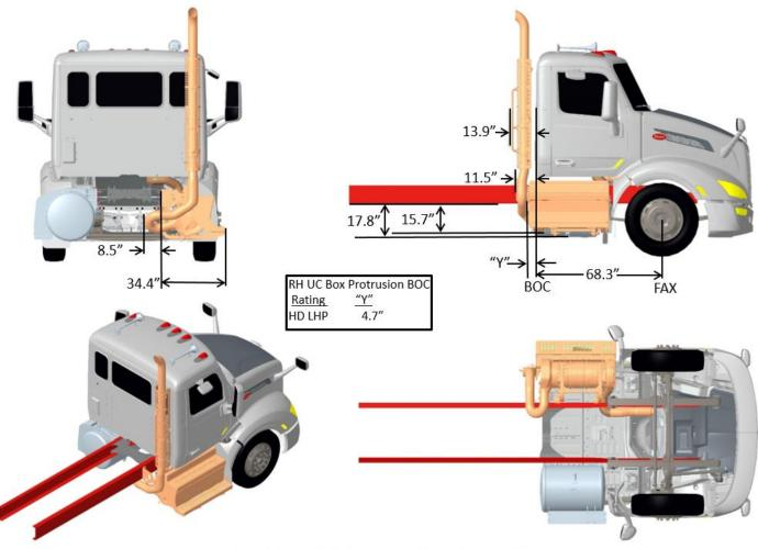
Exhaust Single RH Back Of Cab DPF/SCR RH Under Cab
