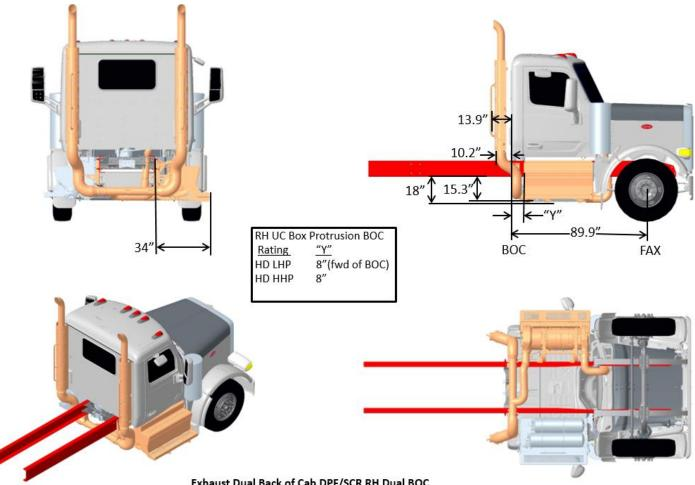
Exhaust Dual Back of Cab DPF/SCR RH Dual BOC
