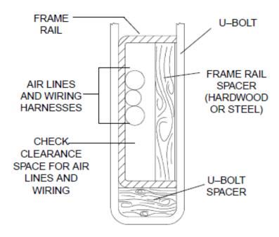
FIGURE 4-10. Clearance Space for Air Lines and Cables
