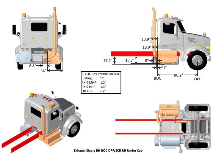
FIGURE 3-49. Exhaust Single RH Back of Cab DPF/SCR RH Under Cab
