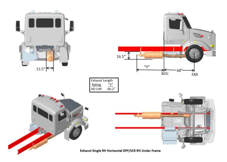
FIGURE 3-45. Exhaust Single RH Horizontal DPF/SCR RH Under Frame
