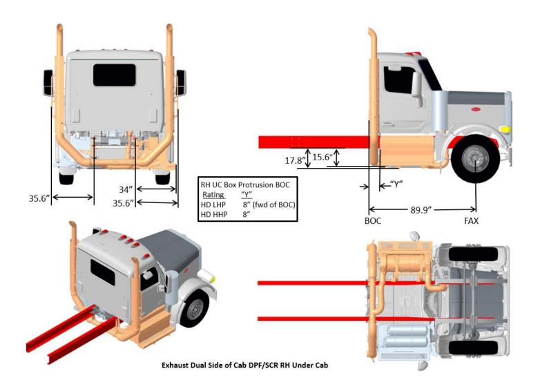
FIGURE 3-34. Exhaust Dual Side of Cab DPF/SCR RH Under Cab (functioning)
