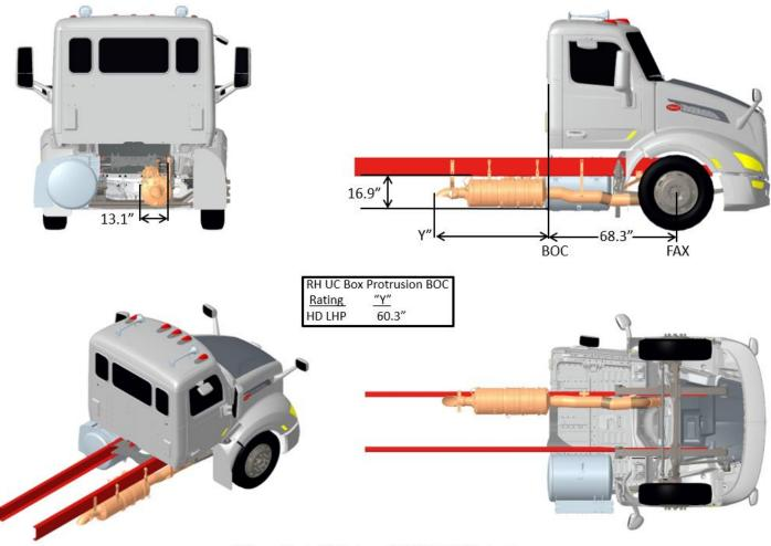
Exhaust Single RH Horizontal DPF/SCR RH Under Frame
