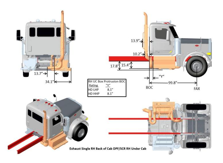
FIGURE 3-36. Exhaust Single RH Back of Cab DPF/SCR RH Under Cab
