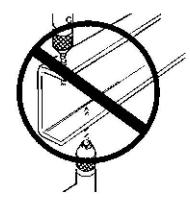
FIGURE 4-8. Frame Rail Flange Drilling Prohibited
