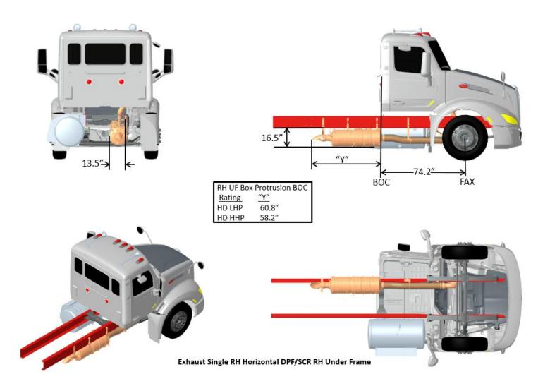
FIGURE 3-80. Exhaust Single RH Horizontal DPF/SCR RH Under Frame
