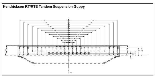
FIGURE 3-23. Hendrickson RT/RTE Tandem Suspension Guppy
