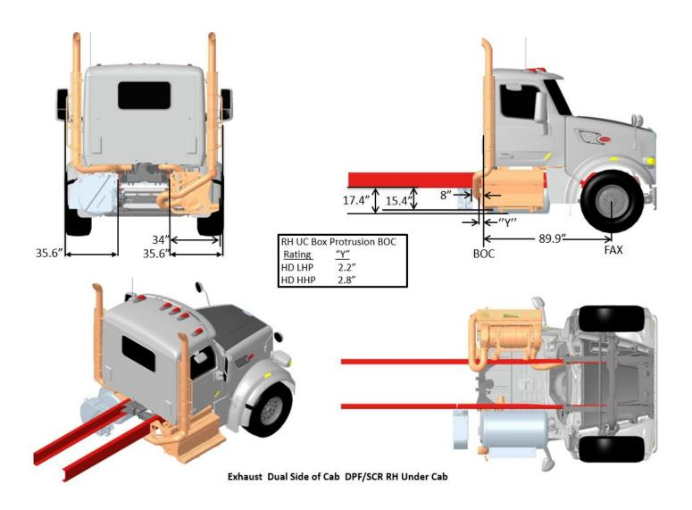
FIGURE 3-68. Exhaust Dual SOC DPF/SCR RH Under Cab
