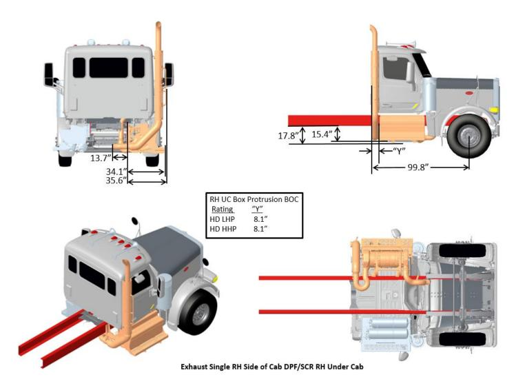
FIGURE 3-37. Exhaust Single RH Side of Cab DPF/SCR RH Under Cab
