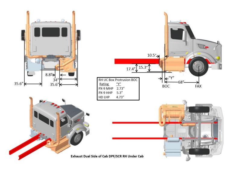
FIGURE 3-46. Exhaust Dual SOC DPF/SCR RH Under Cab
