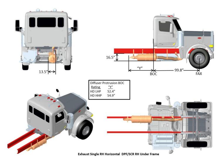
FIGURE 3-39. Exhaust Single RH Horizontal DPF/SCR Under Frame
