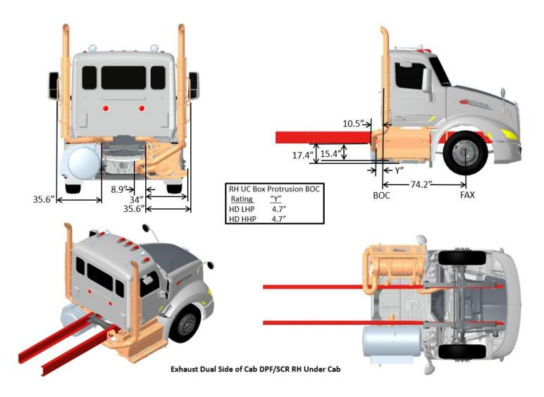
FIGURE 3-81. Exhaust Dual Side of Cab RH DPF/SCR RH Under Cab
