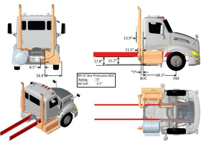
Exhaust Dual Back Of Cab DPF/SCR RH Under Cab
