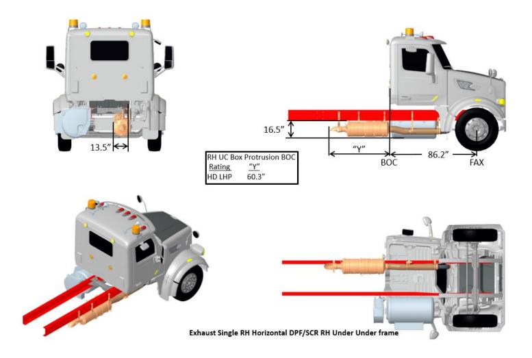
FIGURE 3-52. Exhaust Single RH Horizontal DPF/SCR RH Under Frame
