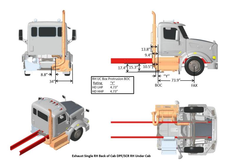
FIGURE 3-56. Exhaust Single RH Back of Cab DPF/SCR RH Under Cab
