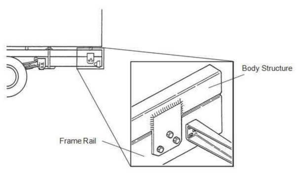
FIGURE 4-11. Fishplate Bracket at Rear End of Body
