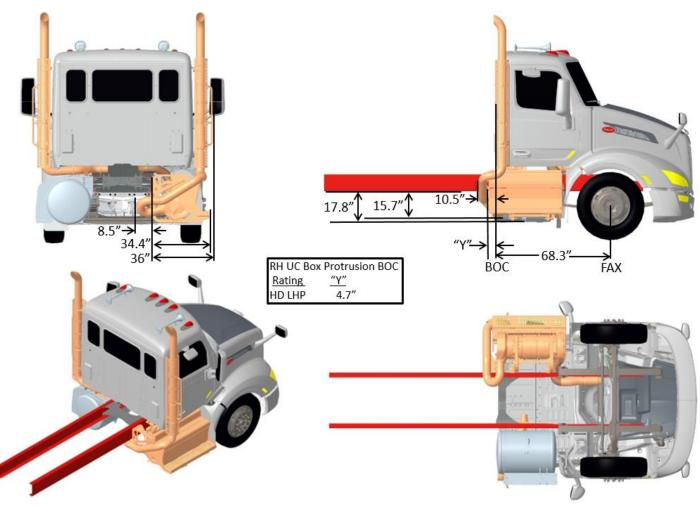
Exhaust Dual Side Of Cab DPF/SCR RH Under Cab
