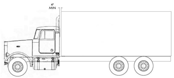
FIGURE 4-2. Minimum Back of Cab Clearance
