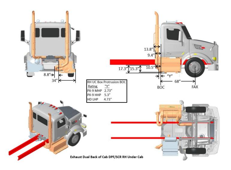
FIGURE 3-47. Exhaust Dual BOC DPF/SCR RH Under Cab
