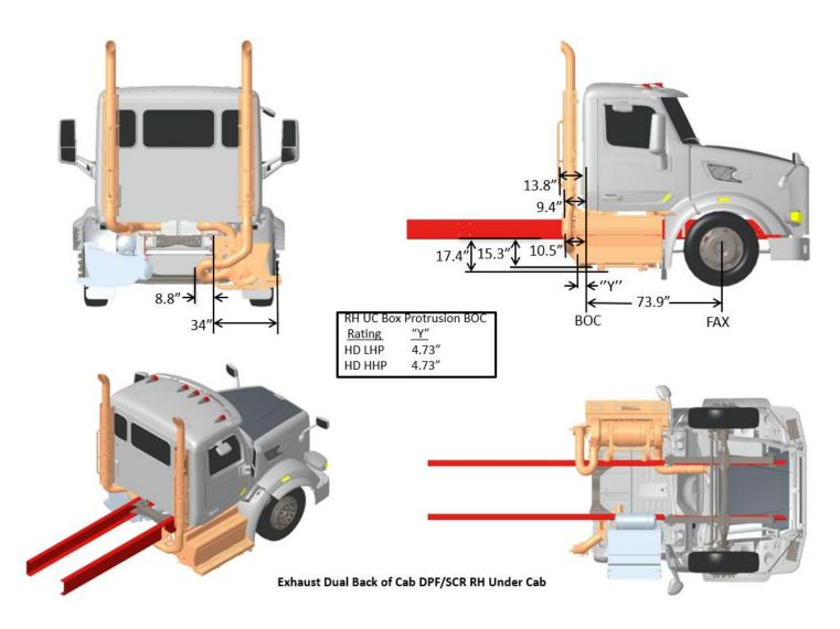
FIGURE 3-62. Exhaust Dual Back of Cab DPF/SCR RH Under Cab
