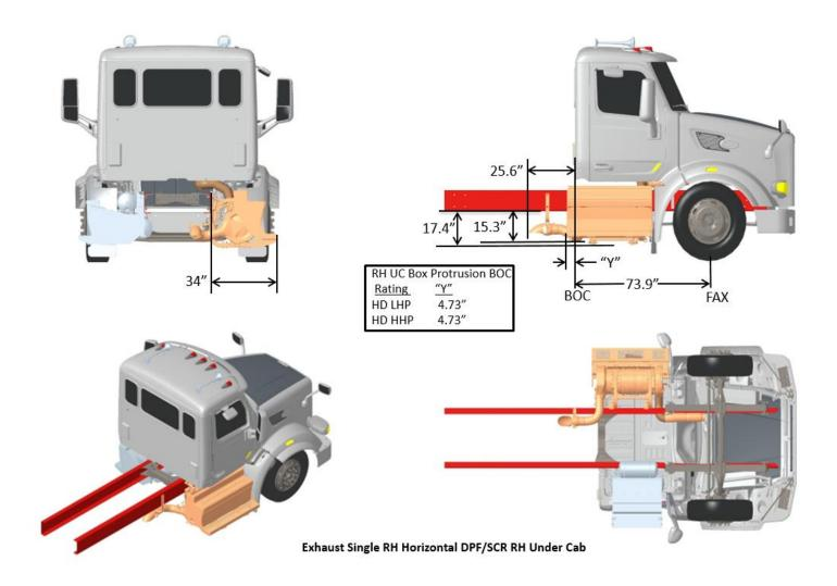
FIGURE 3-58. Exhaust Single RH Horizontal DPF/SCR RH Under Cab
