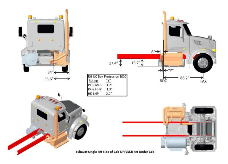
FIGURE 3-50. Exhaust Single RH Side of Cab DPF/SCR RH Under Cab
