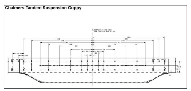
FIGURE 3-20. Chalmers Tandem Suspension Guppy
