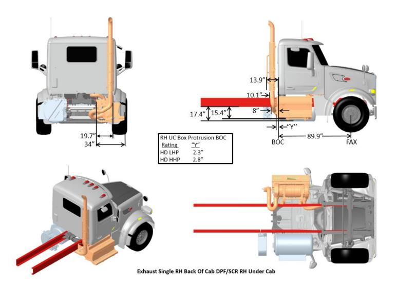
FIGURE 3-63. Exhaust Single RH Back of Cab DPF/SCR RH Under Cab
