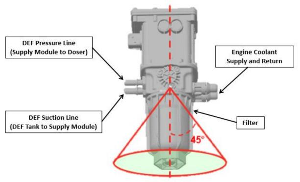
FIGURE 9-4. Supply Module Mounting Angle Limits
