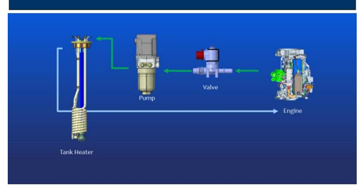
FIGURE 9-1. DEF System Schematic
