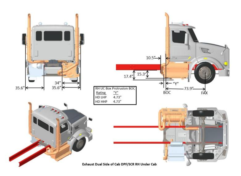
FIGURE 3-60. Exhaust Dual SOC DPF/SCR RH Under Cab
