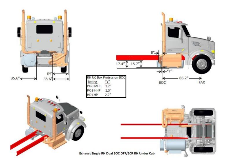
FIGURE 3-53. Exhaust Dual SOC DPF/SCR RH Under Cab
