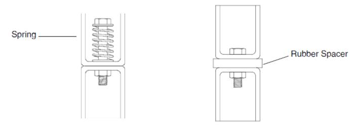
FIGURE 4-4. Mounting Brackets
