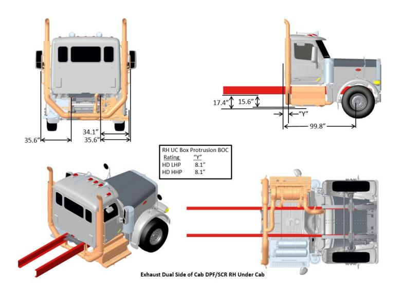
FIGURE 3-40. Exhaust Dual Side of Cab DPF/SCR RH Under Cab (functioning)
