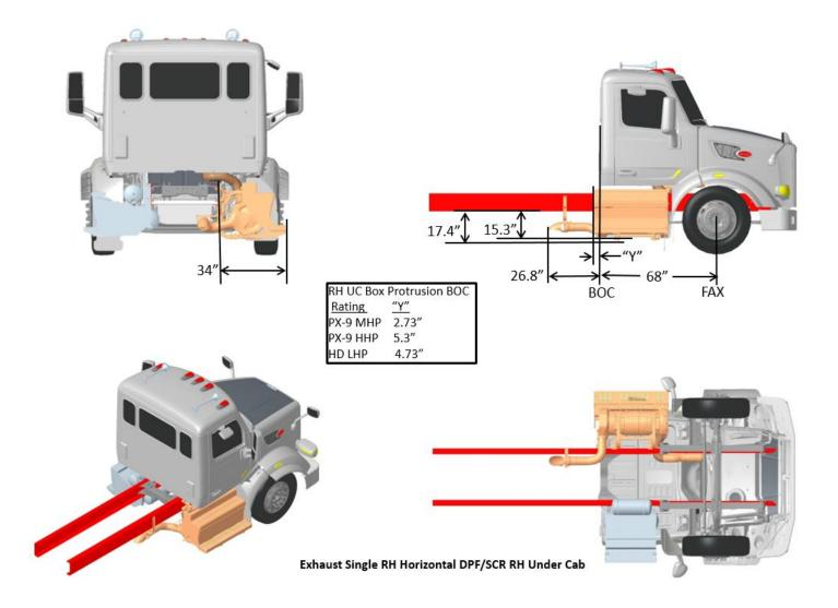
FIGURE 3-44. Exhaust Single RH Horizontal DPF/SCR RH Under Cab
