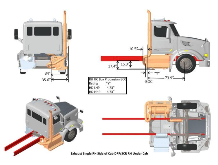
FIGURE 3-57. Exhaust Single RH Side of Cab DPF/SCR RH Under Cab
