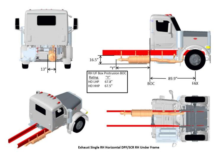
FIGURE 3-33. Exhaust Single RH Horizontal DPF/SCR Under Frame
