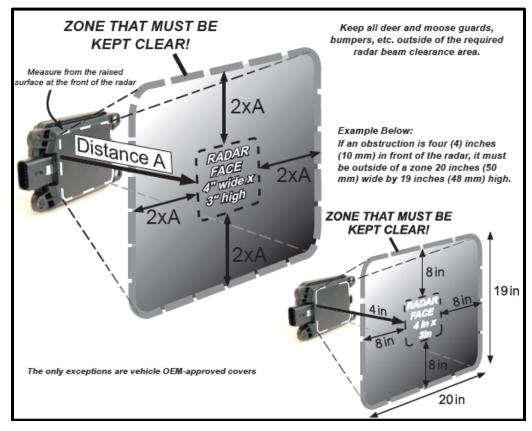
FIGURE 2-5: Fusion 2.0 Radar Clearance
