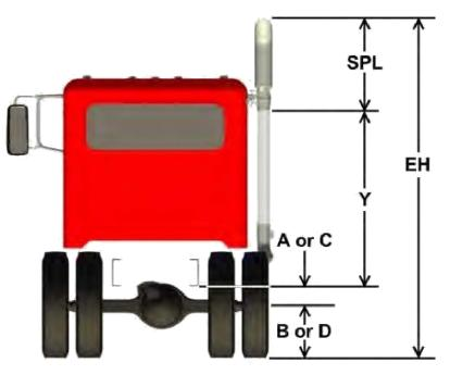
FIGURE 3-25. Exhaust Height Calculations
