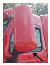
FIGURE 2-3: Aerodynamic Mirror OAT Sensor Location
