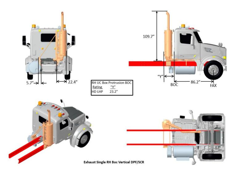
FIGURE 3-55. Exhaust Single RH BOC Vertical DPF/SCR
