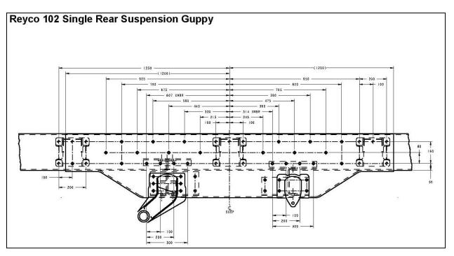
FIGURE 3-24. Reyco 102 Single Drive Suspension Guppy
