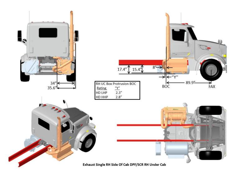
FIGURE 3-64. Exhaust Single RH Side of Cab DPF/SCR RH Under Cab
