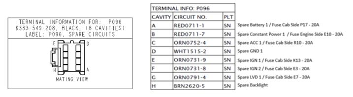
Spare Circuit Connector and Pinout Details
