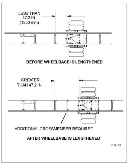
FIGURE 5-2. Crossmember Spacing Requirements
