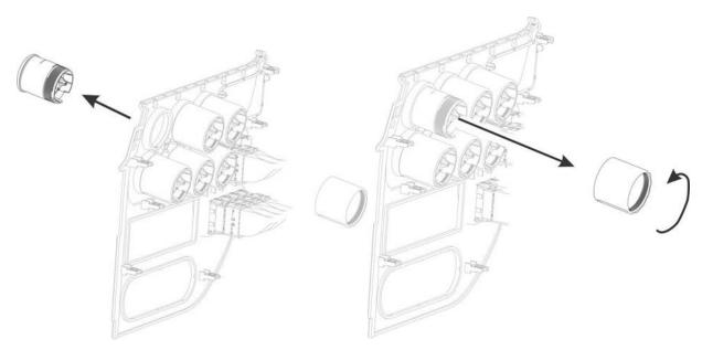
Optional gauges may be installed and connected to the Digital Display via a jumper harness.
