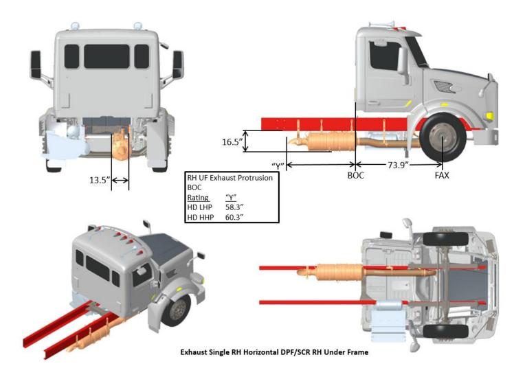
FIGURE 3-59. Exhaust Single RH Horizontal DPF/SCR RH Under Frame
