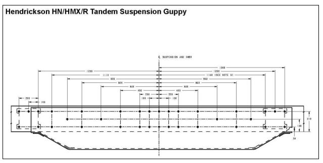
FIGURE 3-21. Hendrickson HN/HMX/R Tandem Suspension Guppy
