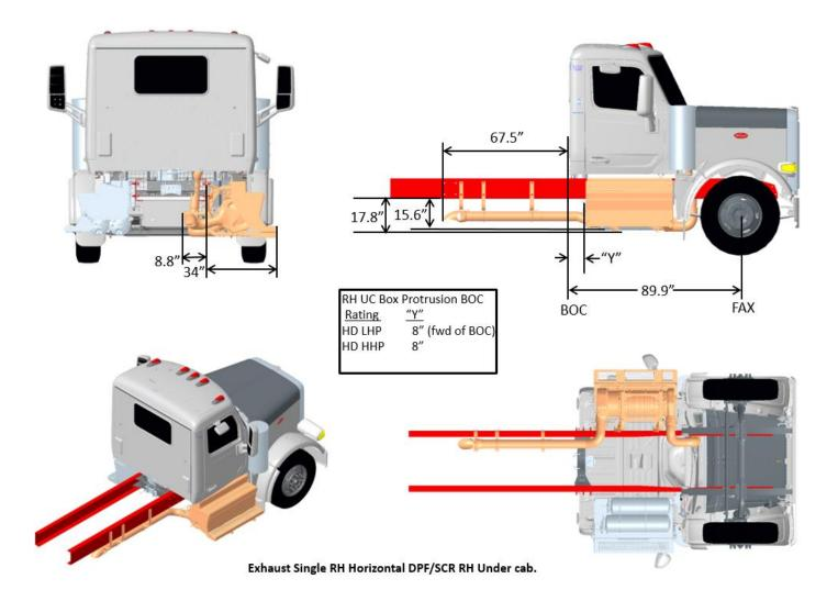
FIGURE 3-32. Exhaust Single RH Horizontal DPF/SCR RH Under Cab
