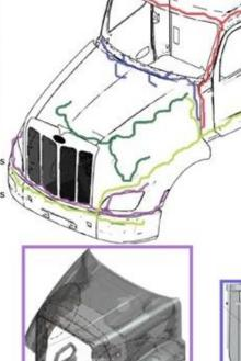
HOOD CHASSIS HARNESS 1) Connections to Main Chassis Harness 2) Connections to Head Lights 3) Connections to Turn Signal Lamps
