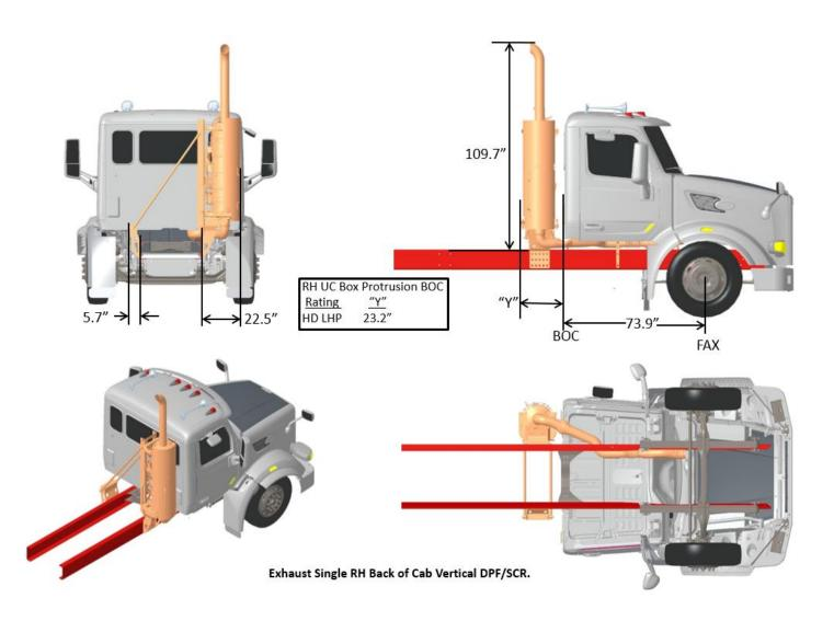
FIGURE 3-61. Exhaust Single RH BOC Vertical DPF/SCR
