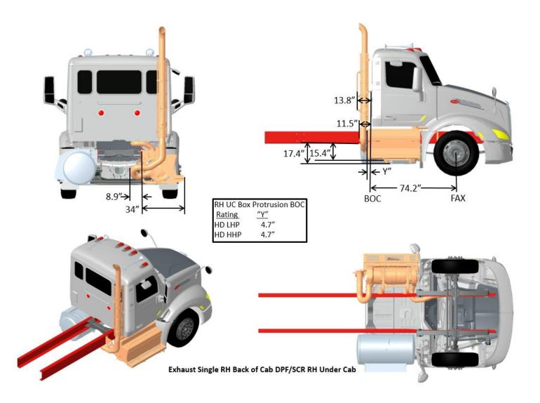
FIGURE 3-77. Exhaust Single RH Back of Cab DPF/SCR RH Under Cab
