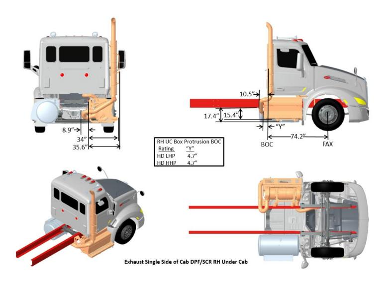
FIGURE 3-78. Exhaust Single RH Side of Cab DPF/SCR RH Under Cab
