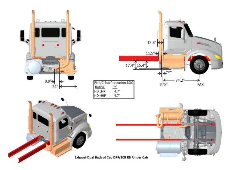
FIGURE 3-82. Exhaust Dual Back of Cab RH DPF/SCR RH Under Cab
