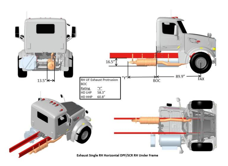
FIGURE 3-66. Exhaust Single RH Horizontal DPF/SCR RH Under Frame
