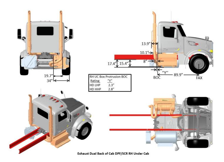
FIGURE 3-67. Exhaust Dual Back of Cab DPF/SCR RH Under Cab
