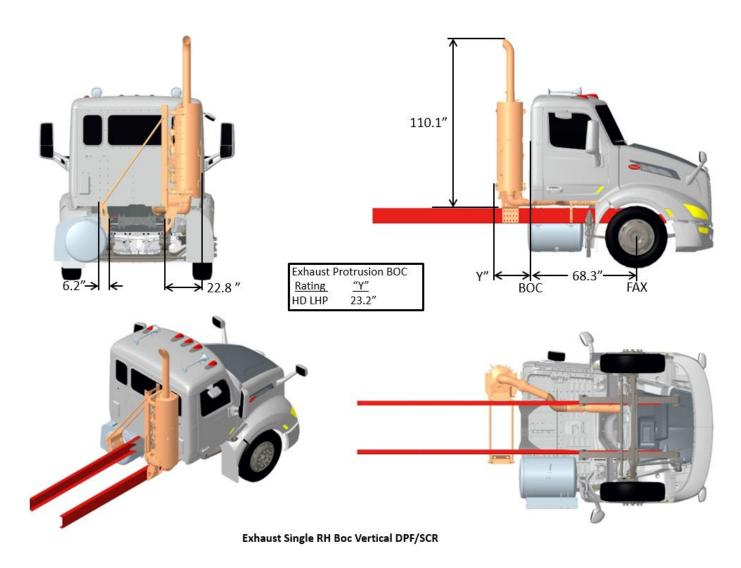
FIGURE 3-76. Exhaust Single RH BOC Vertical DPF/SCR
