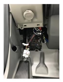
MX PTO CAN functionality may be accessed in the cab through the RP1226 connector and remotely through the body connectors K-CAN (E-3375-021) and B-CAN (DTM06-2S-EP10) Connectors.
