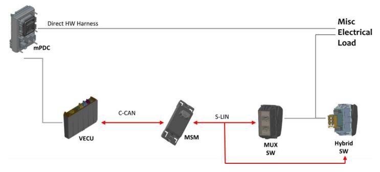
Multiplexing = shorter wire bundles, improved diagnostics, and greater driver feedback. Safety critical switches use hybrid switch with hardwire for redundancy. The switches are less expensive with fewer wires behind the dash and on the chassis. The switches are self-diagnosable to improve troubleshooting with DAVIE. Master Switch Module (MSM) LIN Communication to/from Switches
