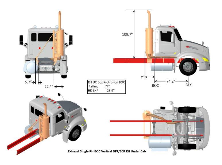
FIGURE 3-83. Exhaust Single RH BOC Vertical DPF/SCR
