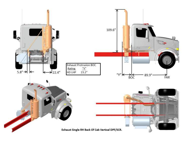
FIGURE 3-69. Exhaust Single RH BOC Vertical DPF/SCR
