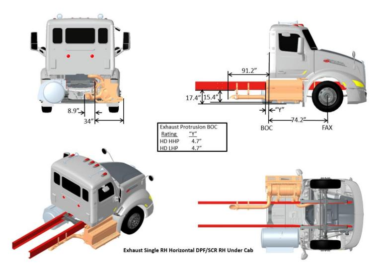
FIGURE 3-79. Exhaust Single RH Horizontal DPF/SCR RH Under Cab
