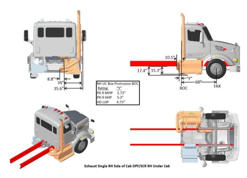
FIGURE 3-43. Exhaust Single RH Side of Cab DPF/SCR RH Under Cab
