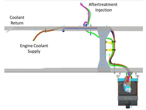
FIGURE 9-3. Routing for DEF and Coolant Lines
