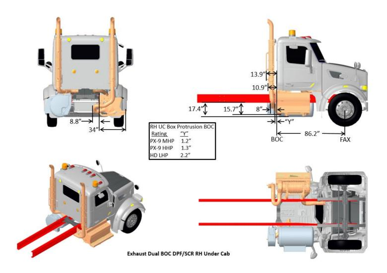
FIGURE 3-54. Exhaust Dual BOC DPF/SCR RH Under Cab
