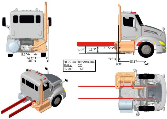
Exhaust Single RH Side Of Cab DPF/SCR RH Under Cab
